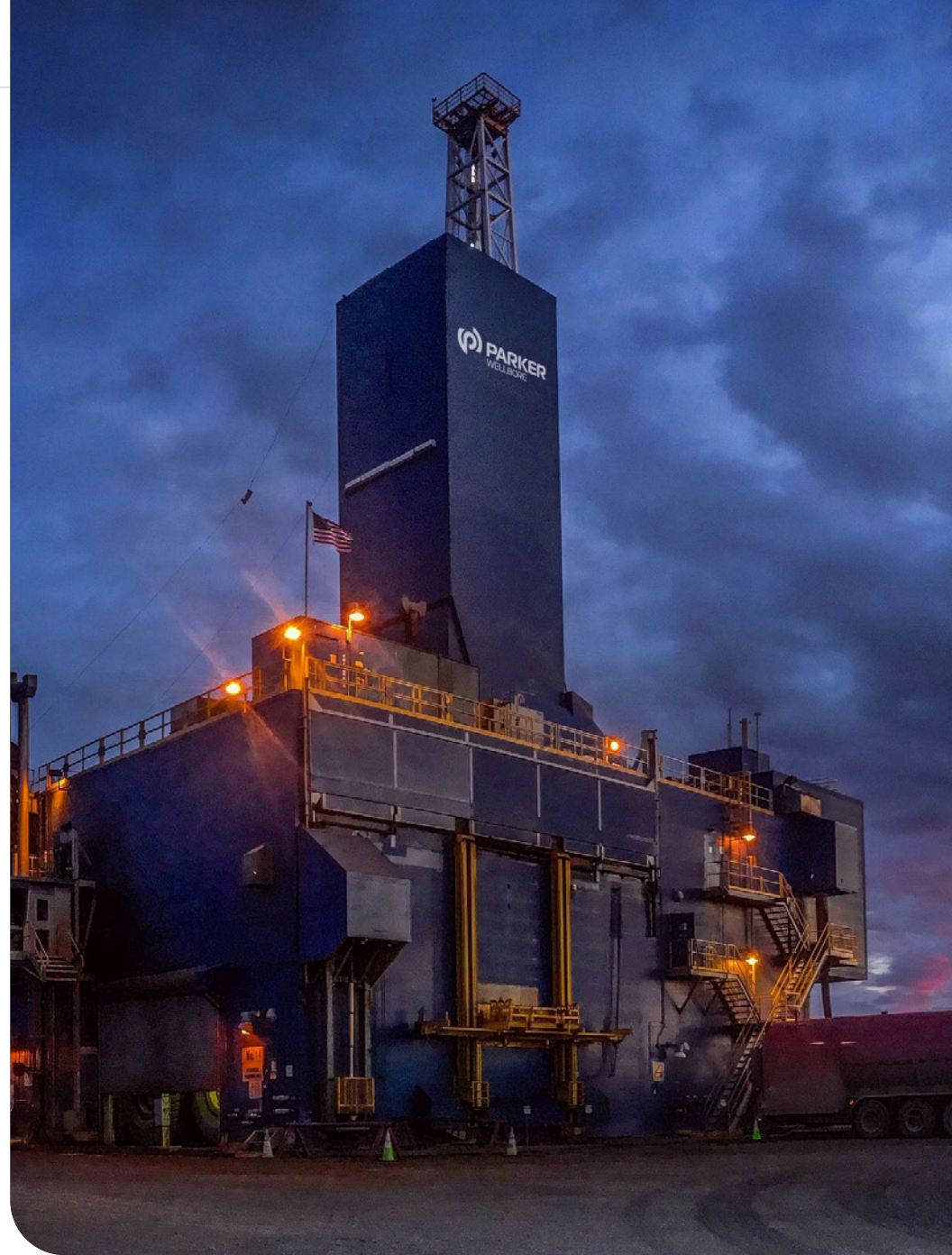
Parker Wellbore Rig 272 is specifically designed to address the many environmental and operating challenges of working on Alaska's North Slope. This rig has the ability to run off highline power when available and EPA Tier IV compliant engines when operating remote.
